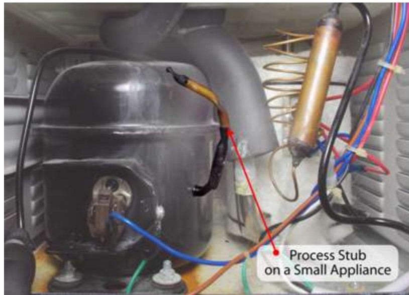
Figure I - 1. Process stub on a small appliance
