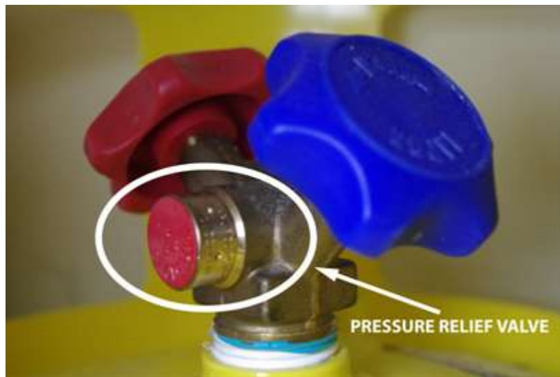
Figure C - 7. Pressure Relief Valve on a Recovery Tank
