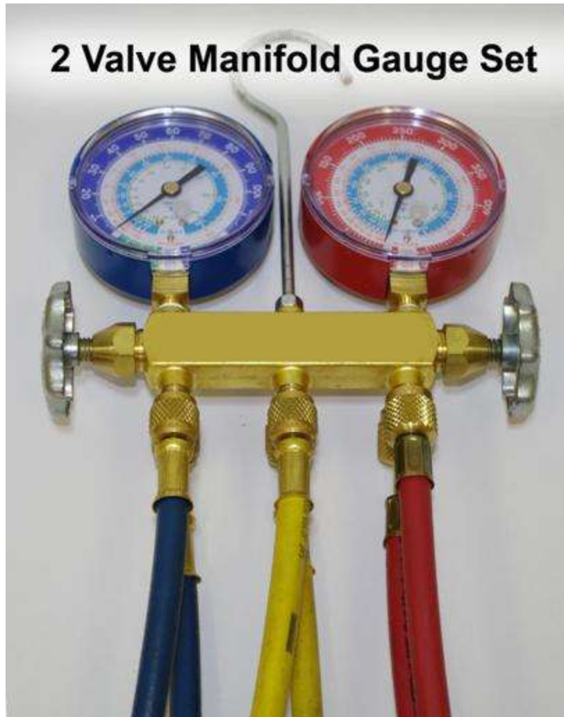
Figure C - 4. Two-valve, three-hose manifold photo
